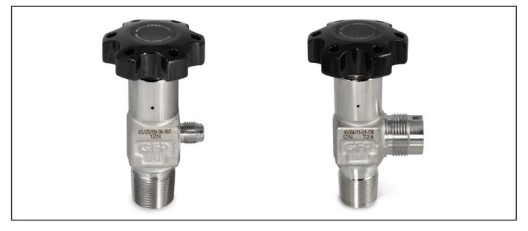
GasFlo Products STA Series Valves are a high pressure, medium flow design. This spring type, diaphragm, forged body, angle pattern valve can be easily field maintained with an economical re-build kit. The STA Series provides an extended service life, positive shut off and smooth operation for pressure ranges from vacuum to 3500 psig.
