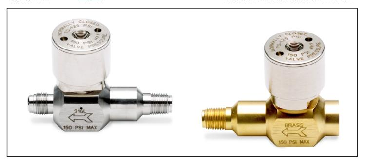
GasFlo Products LPLL Series Valves are manufactured with an extended inlet leg and are air operated to allow for remote automated cycling. This low pressure springless diaphragm design remains closed unless proper actuation pressure is continuously applied. LLPL Series Valves provide superior leak integrity for critical gas/fluid systems with pressure ranges from vacuum to 150 psig.
